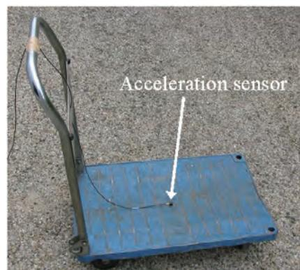
Fig. 3 Position of acceleration sensor.
